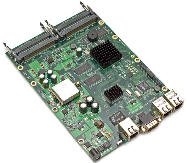
miniPCI slots, three Gigabit ethernet ports and two CF slots for storage expansion. As an added bonus - it also supports daughterboard expansion, including addons made for RB532
