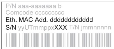
You are also advised to write down the Serial Number and MAC address of the ORiNOCO PC Card(s) that you use with your AP-1000 (the information is printed on a small label at the back side of the PC Card).
